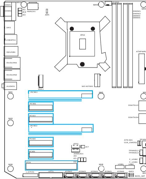
2 x16 slots (2 x16 slots are automatically configured for x8 signals when the remote x16 slot is inserted; Proximal PCIe x16 without card insertion) 4 PCIe x4 expansion slots (3 x4, 1 x1), 1 PCI (32bit)
