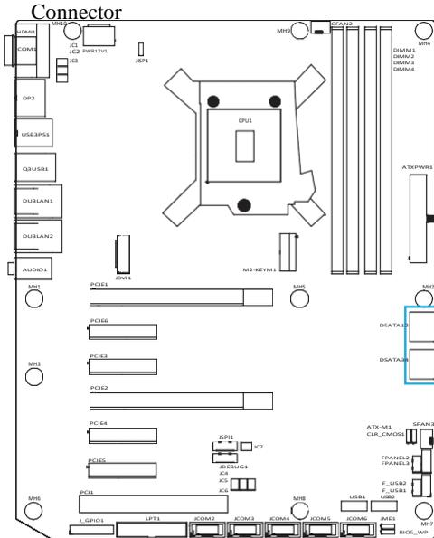
This interface supports the use of Serial ATA cable to connect Serial ATA hard drives or other Serial ATA compliant devices.
