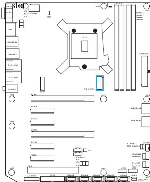
M2-KEYM1 slot, support SSD solid state drive;
