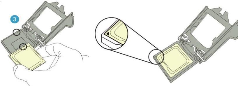
3. After confirming that the CPU has been completely plugged into the CPU socket, put down the pull rod until you hear a light sound of "Ka".
