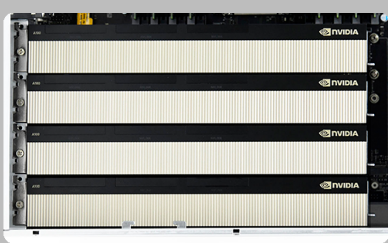
8-slot for 4x GPU Cards
